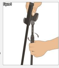
Step 4 – Loosen the knob shown in Figure 4 to adjust the angle of the boom pipe.
