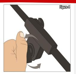
Step 5 - To adjust the boom, loosen the knob located on the left side of the boom and pull or push the boom forward or backward, the tighten the knob to hold in place as shown in Figure 5. This Microphone Stand has an additional telescoping boom located near the microphone. To extend or retract, loosen the knob directly behind the microphone clip and extend or retract the boom (See Figure 6). Tighten the knob to hold it in place.
