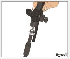
Step 3 — To adjust the height of the stand, simply loosen the hand knob near the connection of the boom piece then adjust up or down the inner pipe to your preference and tighten to hold in place (see Figure 3).
