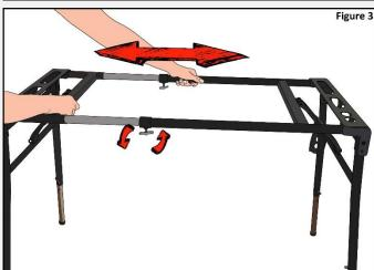
Step 3 - Locate the pair of arm attachment brackets (Part C). Take 1 and place the bracket with 2 knobs (Part D) on crossbar and tighten the knobs as shown in FIGURE 4. Remove the remaining knobs on brackets. these Locate the top arms and align the holes in the arm to the bracket. Insert the knob and put the spring back over the knob. Then screw the knob back into the bracket.
