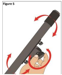
**Step 5** – Loosen the small knobs on the arms to adjust the arms forward and backwards as shown in FIGURE 6. Tighten the knobs when your desired adjustment is achieved.
