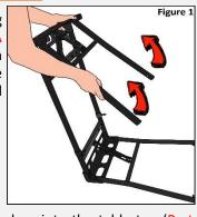
Step 2 – Insert the chrome legs into the table top (Part D). Extend the legs to the desired height and screw the knob (Part E) into the threaded hole as seen in FIGURE 2. If the table is slightly off level, you can unscrew the feet to make the table level. Extend the table to your desired width and lock into place by tightening the knobs as seen in FIGURE 3.
