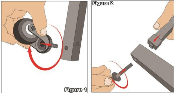
**Step 2** – Take the cross-member bar (Part B) and connect to the bottom support bar (Part A). These has locking clamps that fits through the holes of the bottom support bar and fix in place with a bolt (See above **Figure 2**).
