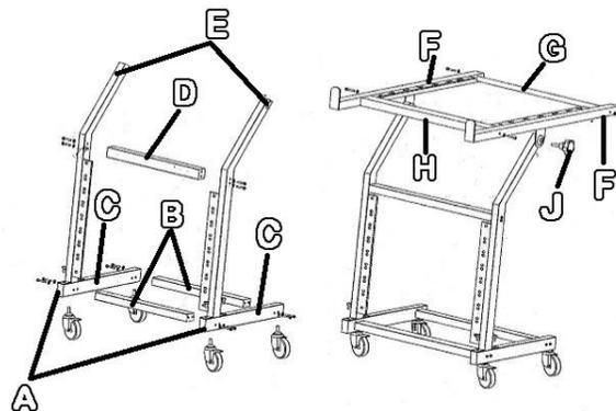
Please note that hardware bolts to assemble the stand maybe screwed into the parts themselves. So, for example, if you are missing a bolt that goes into the bottom base support tube, then look at the end of the bottom base support tube and you will see that hardware bolt is already screwed into the stand. All you
