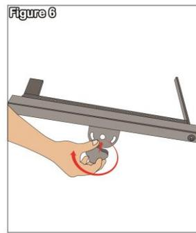
**Step 5** – Now take the piece assembled in Step 4 and place over the piece assembled in Step 3 and secure using a bolt screwed in the center shown in **Figure 6** above.
