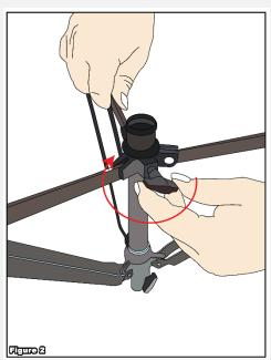
Step 2 – Insert the center post through the bottom of the saddle seat and tighten the knob to keep in place. Also, you need to check the bolt (as seen on Figure 3) and make sure it is tightened well by using an allen wrench.
