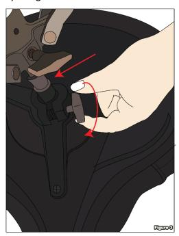
Step 3 – The knob near the center post is to tighten or loosen the spinning inner post with makes the seat swivel, you may or may not adjust this depending on your preference. If you do not want the seat to swivel just tighten the knob (refer to Figure 4). To raise and lower the seat just loosen the knob and turn the seat.
