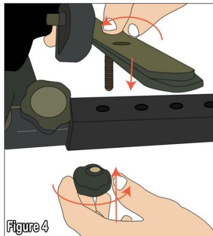
**Step 6** – For safety reasons, please always make sure to test the stability and safety of the product before use. Double check all nuts and bolts, knobs and connectors, make sure that these are tight and securely fastened before use of your product. Test the product under light use or light loads the first time to confirm assembly and structure of the product is correct.
