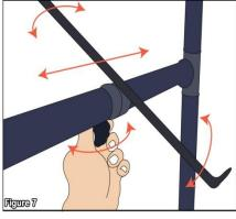
**Step 6 – Figure 7** above shows how to adjust the bracket mounts. It can be adjusted side to side and angled. Once you find you preferred distance and/or angle screw the knob below the bracket mount to keep your setting. The padding on the bracket mounts may or may not be present, if not find the padding in the package and stick it on the bracket mounts. This will protect your equipment and the bracket mount from being scratched.
