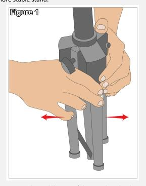
Step 2 – On the middle part of the stand is a knob, turn to loosen and the middle pipe can be adjusted to preferred height. (See Figure 2) Just below the knob is a coupler with a bolt, which may or may not come loose right out of the package, make sure that this bolt is tight before going to step 3.
