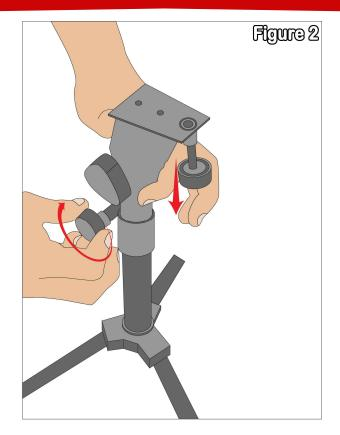
**Step 3** – At the top of the stand is a knob which is the adjustable tilt section of the music stand, adjust to preferred angle and slide the wood plate's bracket and tighten the small screw knob to keep the wood plate in place securely. (See Figure 3)
