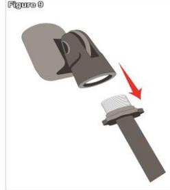
**Step 6** – **Figure 9** above shows how to screw in the microphone clip. Use a microphone clip or shock mount to mount your microphones.
