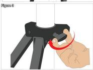
Step 2 – Take the handle and place it on the side of the cranks, there should be a protruding screw to screw in the handle, use the wing nut to secure the handle in place (See Figure 4).
