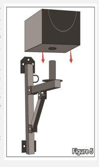
Always check the integrity of the speaker wall mount bracket before mounting anything. You may hold onto the speaker post mount and grip it tightly and wiggle the brackets to test.
