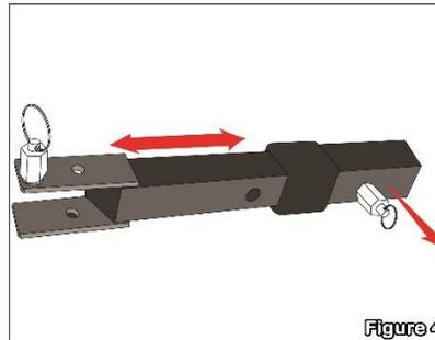
**Step 4** – At the top of the chrome center piece another locking pin (L) is located pull and place the top mount (A). Insert the knob nut (D) and the knob handle (C) on the other side then adjust to your preferred angle and tighten. Once you reach your preferred angle turn the locking pin to secure the angle. (see **Figure 5** & **Figure 6**)
