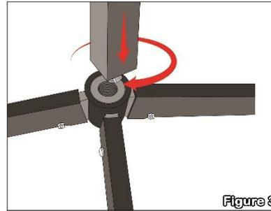
**Step 3** – Take the chrome center piece (I) that goes in the main post, pull the locking pin (J) and insert the chrome center piece. Make sure that the holes in the chrome post align with the locking pin, turn the locking pin (you will hear a click sound) to lock it in place. For additional security of the product tighten the knob (J) on the main post (see **Figure 4**).
