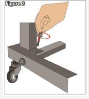
support bar angles out. Screw this in tightly and set aside.
