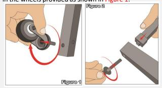
Step 2 – Take the cross-member bar (Part B) and connect to the bottom support bar (Part A). These has locking clamps that fits through the holes of the bottom support bar and fix in place with a bolt (See above Figure 2).
