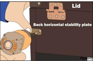
**Step 5** – Turn the stand to the side, at the base (Part A) measure and divide to three sections. Measuring from the front, the leading edge of the bracket closest to the front should be 6" (15.2cm) and the leading edge of the bracket closest to the back should be 13" (33cm). This is where you will drill and screw in the L-Brackets. Do the same step on the other side as seen on Figure 9. Also, while the stand laying on one side you can install the chrome corner brackets as shown in Figure 10.
