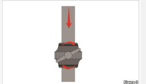
Step 3 – Take the boom arm align the teeth against the top of the middle section, also add pressure since the spring needs to be in the center and use the turning knob to tighten. Once this is in place the boom arm can be adjusted (See Figure 4 and 5)
