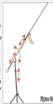
To ensure stability make sure the front of the boom is placed over a leg of the tripod. This type of microphone boom stand comes with a counter weight. If your stand is wobbly or unstable, make sure that the legs are spread wide or adjust the boom arm the opposite way and bring down the height.
