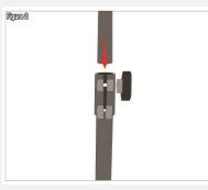
**Step 3** – Take the boom pipe and unscrew the knob so that the boom pipe can be adjusted through as shown in Figure 3. Tighten the knob back to secure (See Figure 4).
