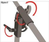
**Step 5** - Take the tip of the boom pipe (extension) and insert through the pipe of the boom, this will allow you to mount the mic. Just screw in the mic handle at the tip as shown in Figure 8.
