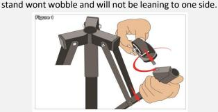
Step 2 – Turn the stand right side up and slide the middle pipe through the middle. Secure this by turning the knob on the shaft. (See
