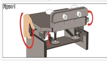
**Step 3** – The pedal extensions are the two rods with a round base and a knob holding the rods. You will see this on the underside of the pedal extender. To adjust this as shown in Figure 2, loosen the knob and make sure that the round base is touching the piano pedals itself.
