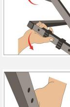
Step 2 – To adjust the height of the stand, each bottom of the legs has a silver push pin that is pushed to allow the slots of the legs to adjust. Pushing or pulling the bottom part will be the height adjustment, if the pin is on the 3rd hole of one leg make sure that all the other pins are on the 3rd hole as well on the other legs. Refer to Figure 2.
